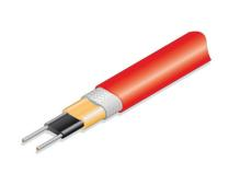
**FSE2-CT, FSEw2-CT** self-regulating heating cable, of **17 W/m, 31 W/m, 45 W/m** and **60 W/m** output for heating and frost protection of industrial pipes, can be installed in both, safe and hazardous (Ex) areas. The cable is produced by nanotechnologies, ensuring long-lasting benefits, withstands the temperature of **up to 100 °C** (swithed ON or OFF).
