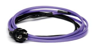
**PipeHeat-10** is a self-regulating heating cable with a plug, of **10 W/m** output, and Adflex (polyolefin) overjacket. **PipeHeat-10** can be installed directly on a pipe's surface or inserted into pipe through a metal fitting otherwise.
