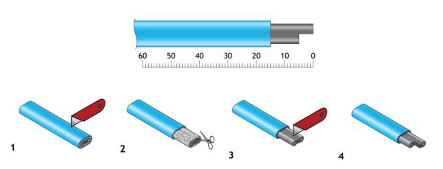
Measure 60mm from end of cable Using a stanley knife, cut away 5mm of and using a stanley knife, score one conductor through the insulation Self-regulating cable is ready for the end seal. around outer jacket, and remove the screen.
