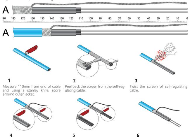
Using a stanley knife, score and peel the self-regulating cable isolation.
