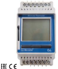
**ETN4-1999** is an electronic thermostat with LCD display, temperature differentials adjustment, independent control relay, and DIN rail - mounted contacts built in a panel. The thermostat made to control both, heating or cooling systems, with support of one or two sensors. The thermostat comes with **ETF 144/99** sensor.
