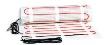
CSCV-150 is a single conductor heating mat of  $150~W/m^2$  output, with extra aluminium foil braid, drainage wire and tinned copper screen and fibreglass mesh. It is self-adhesive on the concrete
