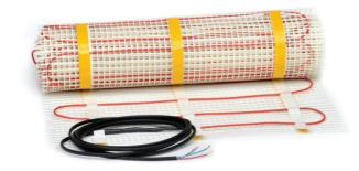
CTAE-160 is a twin conductor heating mat of 160 W/m² output, with extra aluminium foil braid (with memory), drainage wire and fibreglass mesh. It is self-adhesive on the concrete base. Greenline design, the environmentally friendly heating mat, has no lead.
