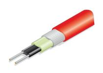
**FSM2-CT** self-regulating heating cable of **11 W/m** and **17 W/m** output can be used for heating, temperature maintenance and frost protection of pipes. The cable is produced with nanotechnologies, ensuring durable benefits; it withstands the temperature of **up to +85 °C** (switched OFF). It can be installed in residential, public and commercial buildings and within industrial hazardous (Ex) areas.
